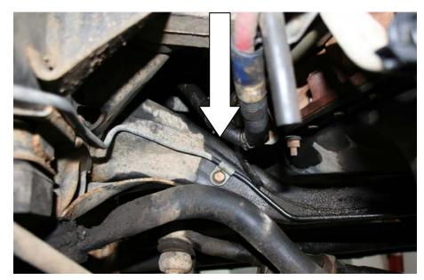
Insert tapered insert (#1302042Z) into the driver's side track bar mounting hole.
