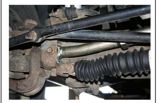
On the driver's side use the 14mm bolt and hardware provided to secure the track bar.
