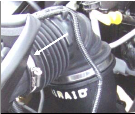
13. Slip the intake tube onto the air filter adapter, and tighten the clamp.
