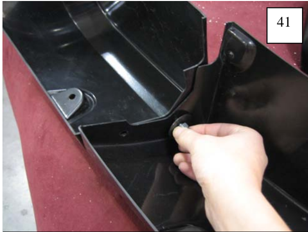
Slide a supplied Large Washer onto backside of bolt, and thread a supplied Nylock Nut onto bolt. Using a 10mm socket and 7/16" wrench, tighten bolts.
