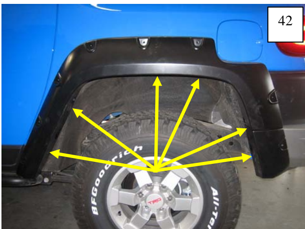
Position Flare on fender. Install six supplied #14 Hex Head Bolts. Do not tighten. NOTE: It is helpful to install one of the top screws first.
