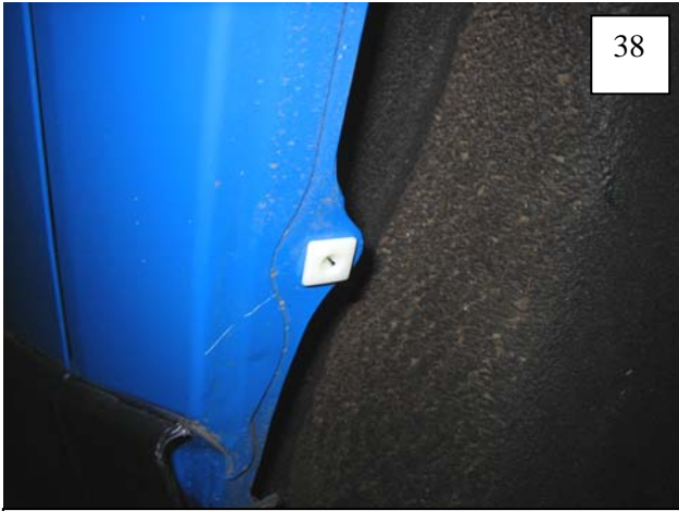
Install a supplied plastic grommet in square hole at front of wheel well.
