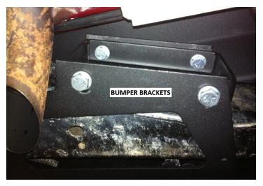
the mounting bolts starting with the lower extended section of the bumper bracketry. Torque the frame bolts and frame box hardware to 80-100lbs.
