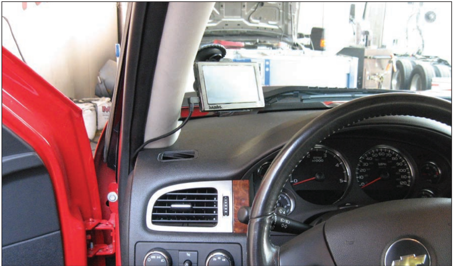
Figure 4 Suggested Mounting location for Banks iQ, Chevy LMM Shown
