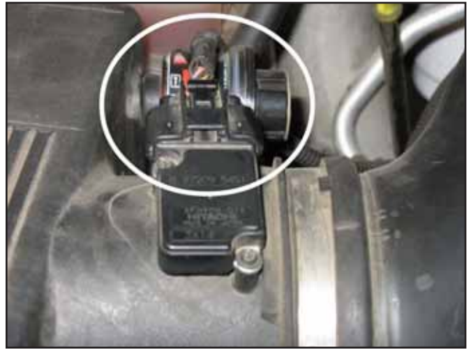
b. Unplug the mass air flow (MAF) sensor wiring harness.
