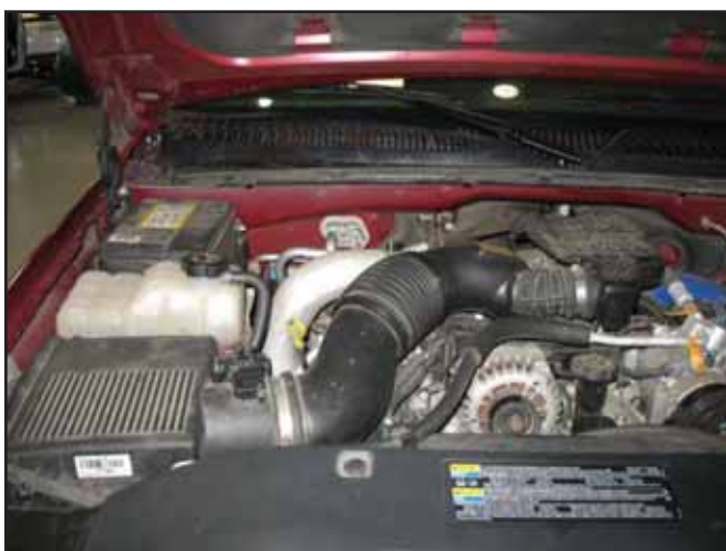
Factory air box system installed
