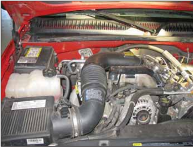
Factory air box system installed
