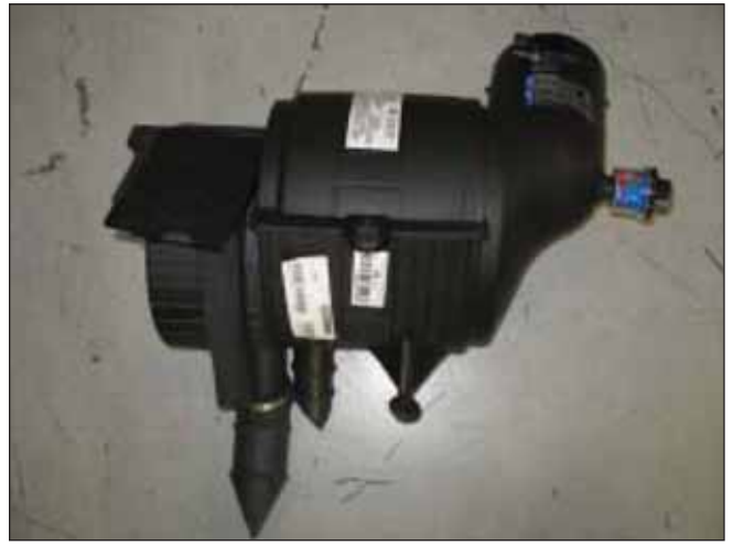
d. The air filter housing is held in place by two grommets on the mounting plate. Gently lift up on the air filter housing and remove it from the engine bay.
