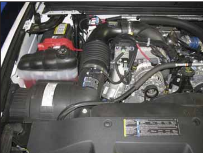
Factory air box system installed
