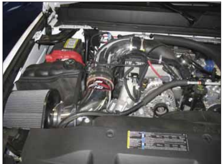
AEM® intake system installed
