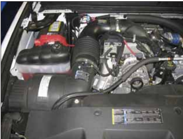
c. Loosen the hose clamps on both ends of the inlet tube. Remove the inlet tube from the engine bay.
