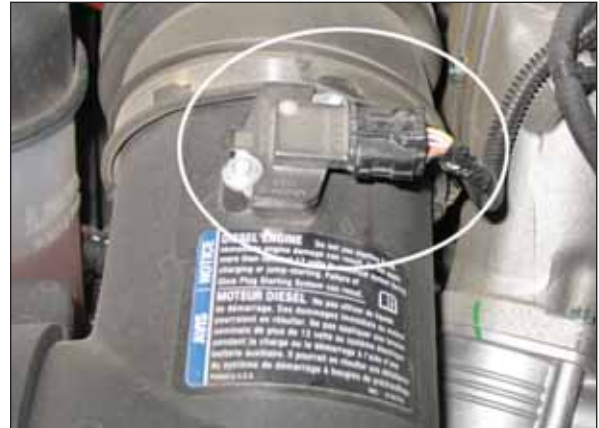
b. Unplug the mass air flow sensor (MAF) wiring harness.
