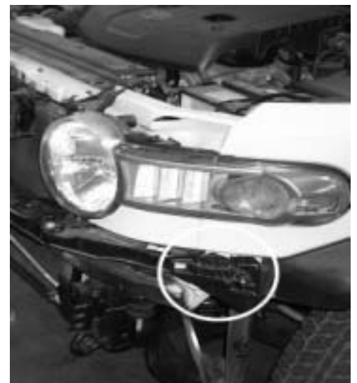
Photo 5 - Outer bumper support clips. These must be removed from both sides.
