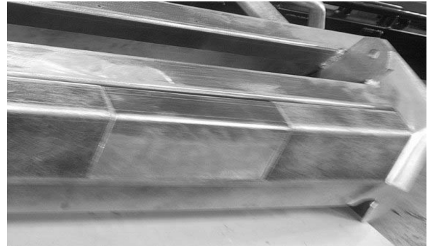
Photo 5 - Fairlead slot cover plate installed
