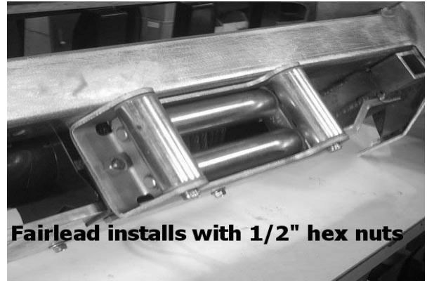
Photo 3b - Roller fairlead installed
