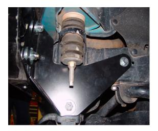
The rear most hole of the bracket uses the small .75"x3" sheet metal piece with the "nut-insert" in it, and a 3/8" x 1.25" bolt with washer. Note: the direction the face of the nut-insert is away from the frame reinforcement bracket, with the nut facing toward the inside of the Fj cruiser. **Put this piece in first!!!**
