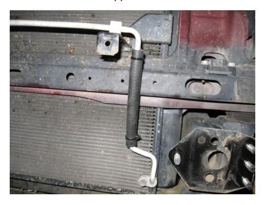
Cut a 6" section of 3/8" fuel line, split down the length and slide over the A/C line carefully. You can use two zip ties or hose clamps to secure. Make sure the hose is situated where the line could rub the
