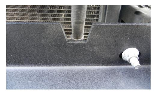
This is a common scenario when installing any aftermarket bumper with a winch mount on an FJ. The easiest way is to modify the mounting bracket as shown below but you may need to take your FJ to an A/C shop to have it moved more. All installations will vary.
