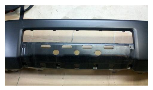
Carefully cut and remove this strip. We suggest leaving 1/2" of material and carefully trimming this back afterward. You can use tins snips, a Dremel or even a hacksaw for this part. (Dremel works best)
