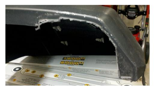
You can lay the bumper cover on the vehicle and against the winch mount to see where it needs to be cut and achieve the correct profile. We use a Dremel and small cut off wheel but you can use whatever you are comfortable with. Trim and cleanup with a razor for a perfect fit. While the cover is on make sure your winch mount is aligned properly.
