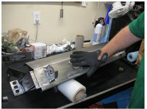
You **must** give it a thorough cleaning using Wax & Grease remover that can be found at any auto parts store in the paint section. This is necessary to remove machine oils and other contaminants that will prevent paint and/or powder coat from adhering to the steel. Make sure you clean every corner and groove.
