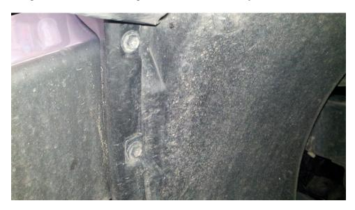
The bumper cover is ready to remove but is still attached via two plastic mounts on the sides underneath the cover. We have found that if you grab the inner fenderwell portion of the cover and pull towards the rear of the vehicle then out to the side it is easier to remove without breaking any plastic mounts. Patience and finesse are key here.
