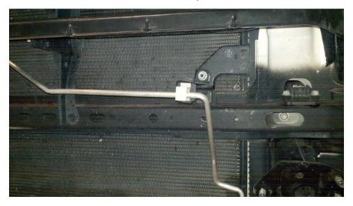
Here is the A/C line. The rear of the winch mount can hit this line if you do not move it and will eventually rub through the tubing if it does make contact.
