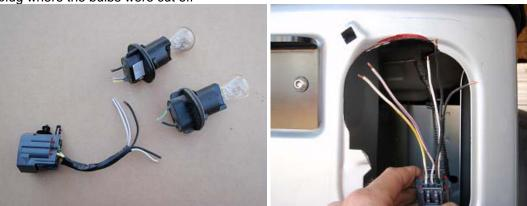
2. Connect your LED light wires to this harness. Below are the wires to join
