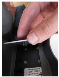
Step 3: Screw plate onto DashDAQ ensuring that the speaker side is up, using the top screw holes. Holes on backer plate should be closer to the top at installation. Do not over tighten.
