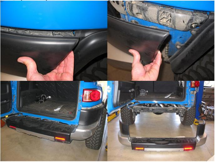
6. Next you must remove the outside "corner pods." To do so you must depress each of the clips holding the corner pod onto the main bumper cover. See photos below for clip locations. Remove both "corner pods." It will look like the last photo (but your cover will be off of the vehicle).
