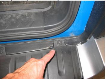
2. Using the tip of a small standard screwdriver, remove the body clip shown below.
