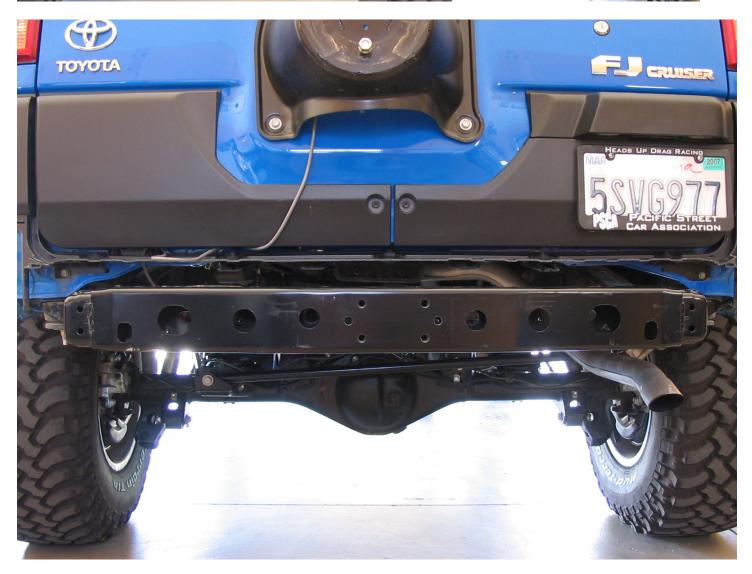
13. Next you will have to slot the bumper cover to allow the frame plates on the bumper (see photo below with arrow) to slide all the way forward. Slot with you hand saw just deep and wide enough to allow the bumper to slide all the way forward and end up against the rear cross member.
