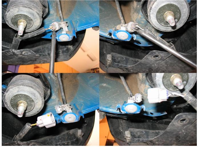
5. With all bolts and body clips removed, carefully pull the forward upper corner plastic away from the body. It is secured with a series of "barbed fittings" that engage with the body and additional plastic on the rear of the vehicle. Pull gently to avoid breaking off these barbed fittings. You will be using them to re-install the plastic after trimming. After the bumper cover is loose, at all points from the vehicle,
