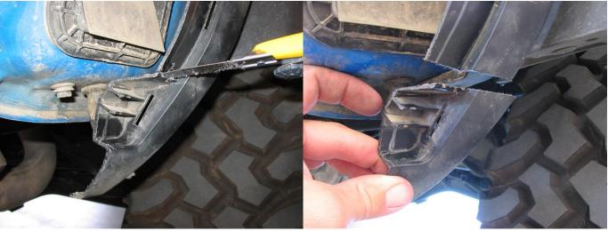
9. Bend the back up sensor wire bracket, upward until it is flush with the bottom of the body. See photos below.
