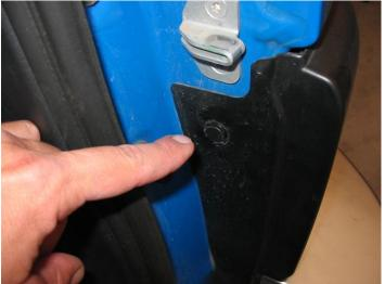
3. Remove the bolts holding the lower edge of the rear bumper cover as shown below.
