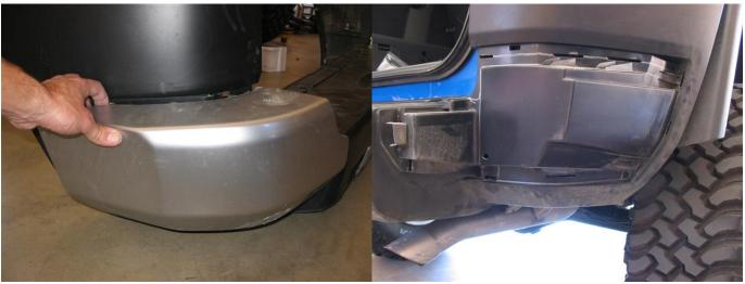
7. Study the below "post trim" photo. Using a marker to create reference marks along the "edges" you will follow with your small hand saw, trim the "corner pod window" out as shown, leaving a 1" lip. Check twice, mark, re-check and finally cut once!!
