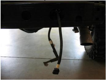
21. Remove the backup sensor from your stock bumper cover by sliding the clip off the sensor on the backside of the cover. Install on your new bumper as per photos below. Re-attach the retention clip on the backside of the bumper.
