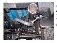
**5.** Next, install the exit pipe #D. onto overaxle pipe. Use clamp #F to secure to the tailpipes. DO NOT TIGHTEN. Insert welded hanger into rubber grommet.
