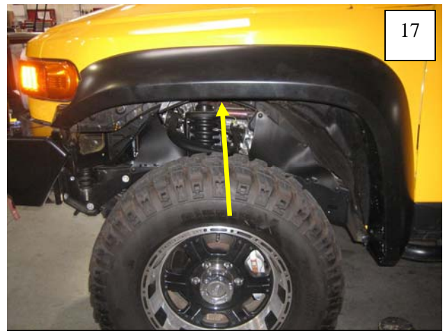
Install one supplied Christmas Tree Fastener in top hole. Check that edge trim is seated correctly, then tighten all bolts.
