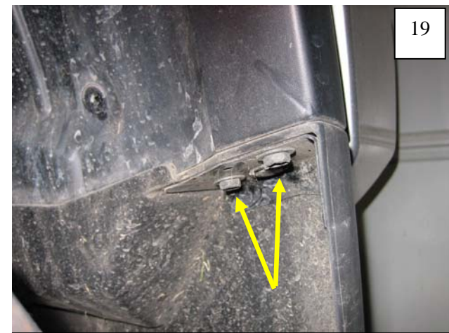
Remove two bolts from mud flap.
