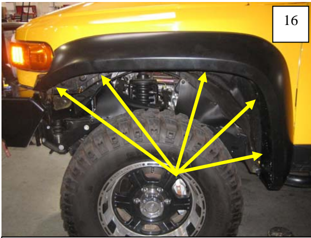
Position Flare on fender. Install five supplied #14 Hex Head Bolts. Do not tighten. NOTE: It is helpful to install one of the top bolts first.
