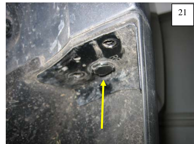
Remove one plastic fastener from mud guard.
