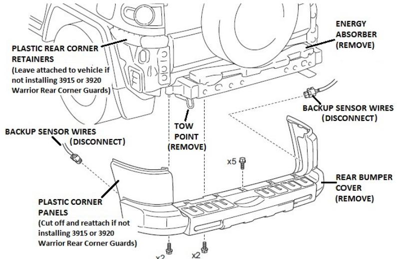
2. Begin removal of the rear bumper cover taking care not to break any mounting tabs of the plastic corner panels. Remove the rear bumper energy absorber, side stays, side support sub-assemblies, rear bumper bar brackets and the tow point.
