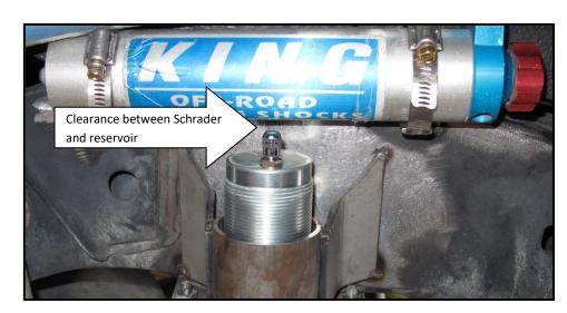
14. Once everything is tacked and clears, weld the bump stop mounts, strike pads, and reservoir mounts, then apply a coat of spray paint.
