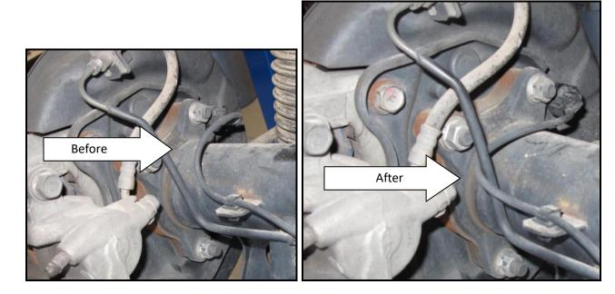
8.Cycle the rear end up to see where the bump is going to contact the axle, mark the axle and clean off the paint so the strike pad can be welded on. If you have access to nitrogen, we recommend letting the pressure out of your bump so you can cycle your suspension all the way up for more accurate strike pad placement.
