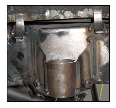
15. When everything is painted and dry, install the reservoir onto the tabs and tighten the hose clamps. Next install the bottom lock rings on the bump stop all the way to the bottom, making sure the set screws are not sticking through the top or the bottom of the ring.
