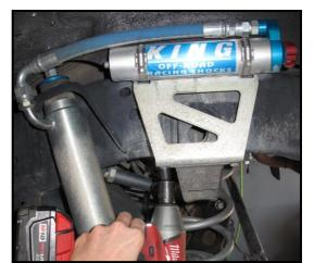
2. With the bracket removed, mark the welded bump stop mount where it needs to be cut on the side of the frame as well as underneath the bracket.
