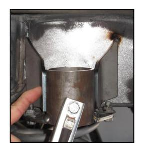
6.Put the new King bump with the lower lock ring bottomed out into the mount, and remove the coil spring from the vehicle.
