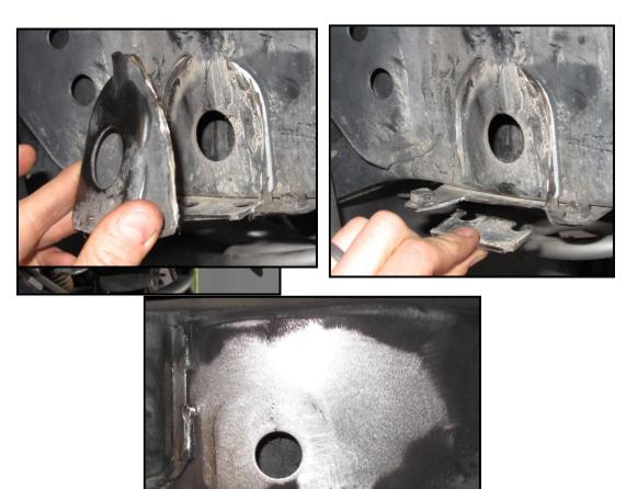
4.Bolt on the supplied bump stop mount using the stock hardware (Note: they are stamped left and right) to the frame.
