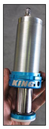
16. Once the bottom lock ring is on, insert the bump into the mount and spin the top lock ring down onto the mount. Use a spanner wrench or a hammer and chisel to lock the top lock ring onto the mount.
