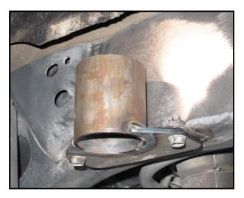
5. With the mount bolted on, place and tack the side plates onto the frame and mount.
