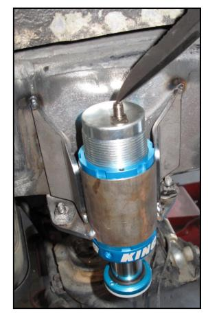
9. After the axle is clean, cycle the axle up, set the placement of the strike pad and tack it in place.
