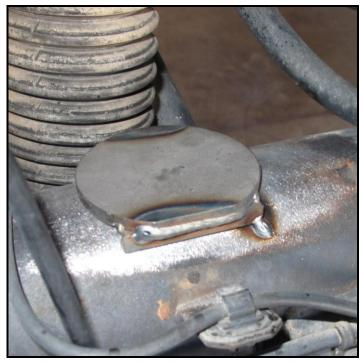
10. Remove the paint from the top edge of the frame so that the reservoir tabs can be tacked in place.
