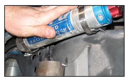
13. Once tacked into place, put the bump stop back in the mount and make sure the Schrader valve doesn't contact the reservoir and has a small gap between the two.
