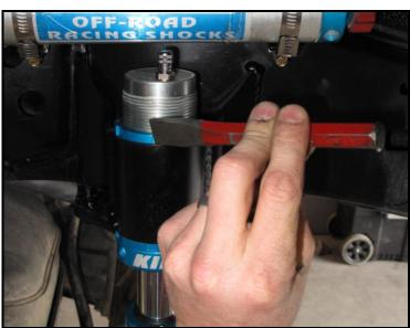
17. Use a 5/32" Allen wrench to tighten the upper set screws on the top lock ring.
