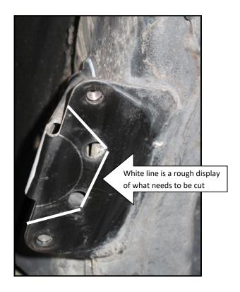
3. Disk cut the mount off and sand the frame clean.
