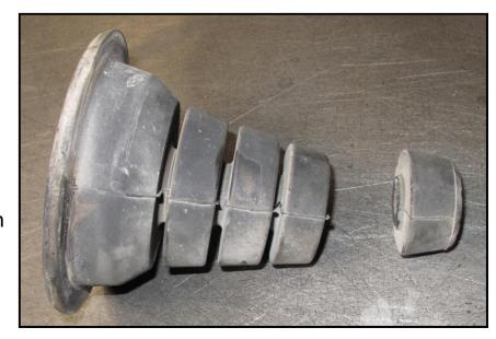
19. Once the bump stop is cut, reinstall the springs, make sure all hardware is tight, re-install the wheels and re check all hardware after 100 miles.
