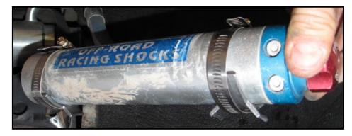
12. Set the reservoir on the top edge of the frame making sure both mounts make contact with the frame, and tack weld the tabs.
