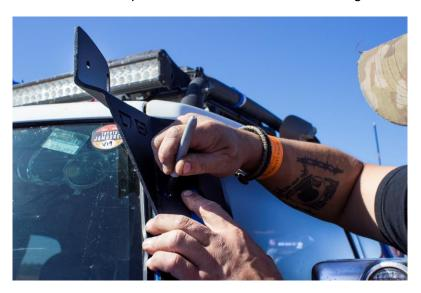
2) Beginning with the top right hole mark, **bore a 1" hole** using the **7/32" drill bit**. Make sure to keep the drill bit straight as you bore the hole.
