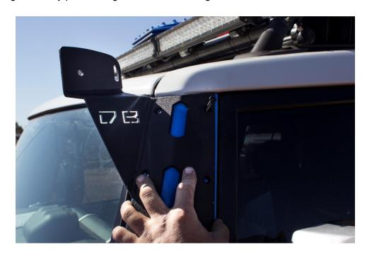
4) With the top screw in and the Light Mount in place, finish drilling the rest of the holes using a **criss-cross motion**, as shown in the picture below.
