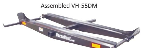
Assembled view from above. Remove Reflector backing and affix Reflectors as shown.
